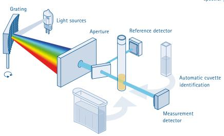
Exact and reproducible measured values: determination of the spectral colour value with a resolution of 10 nm, together with automatic cuvette identification, guarantees unsurpassed measurement reliability. One advantage of the spectral measurement is long-term stability, as, in contrast to filter photometers, no ageing occurs.
