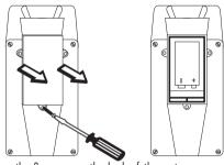
Unscrew the 3 screws on the back of the meter, remove the battery cover and replace the battery while paying attention to its polarity.
