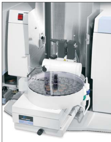
Figure 10. The AS-800 autosampler can accommodate up to 148 samples.
