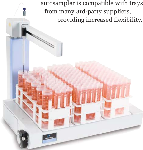
Figure 11. AS-93 plus autosampler for fully automated flame analysis.
