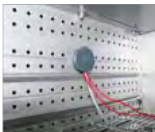
Access port with silicone plug
