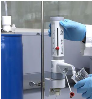
Remote Dispensing System for Drum Dispensing
