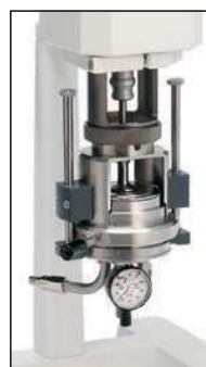
RST-90Y Spindle for BU measurements on joint compound and similar materials
