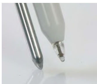
pH tip embedded in break-proof plastic
