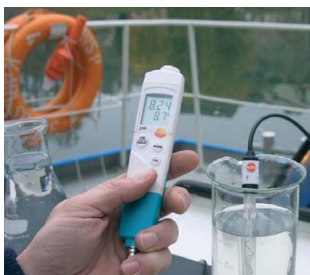
Automatic temperature compensation in external probes with temperature sensor
